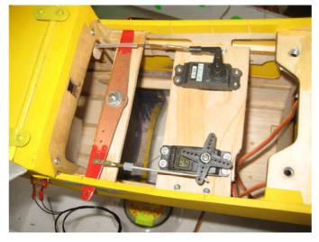
The elevators presented another problem – how to get the exits in the right place and lining up with the servos (I decided to put a servo on each half). I used a bit of tubing inside the fuselage set in a balsa support at the right angle. One curious feature of the
