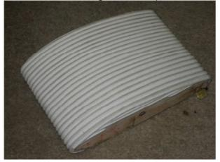
centre of the top wing?" So he told me and very clever too! Stick strips of single core electrical flex around the tank (it has to be good and flexible to go around the LE) and then wipe over with white "No More Gaps". Works a treat, here it is just drying out.
