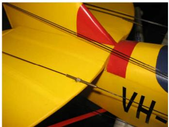
Moth is that the top cables actually rub on the top of the tailplane so the angle has to be just right. They have a small support where they cross the LE and that section is actually a solid rod not cable - I just put a piece of brass tube over the cable to simulate it. The ailerons are easy, just servos in the bottom of the wing direct linked to the horn (more circuit board of course).
